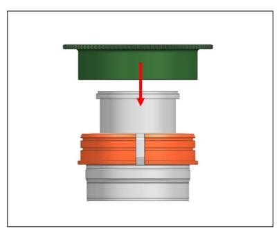
2 Insert the N2450-Z Zoom Gear on the plastic C-ring until it reaches the flange of the plastic C-ring.
