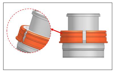
1. Insert the plastic C-ring as shown and place it over the lens.
