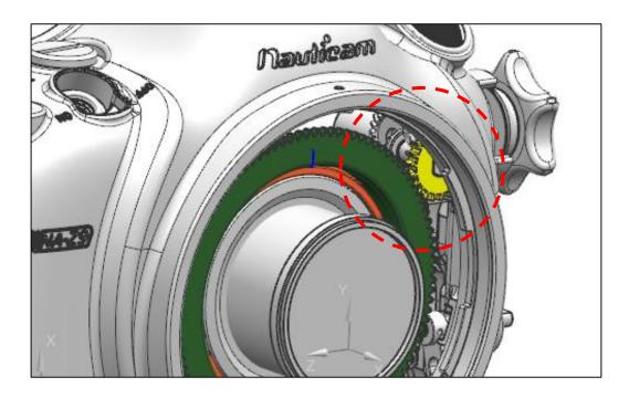
1. The N2450-Z Zoom Gear can be controlled by zoom/focus knob of the housing.
