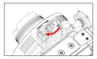
Lift the port lock/ release latch on the other side of the adaptor. Then Press and hold the RED port release safety button, turn the port lock/release latch clockwise until it stops.
