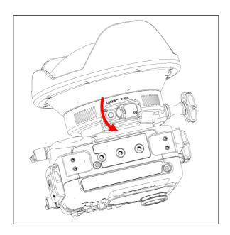
To lock the port in place, turn the port lock/release latch count clockwise to the original position and then flip it down.
