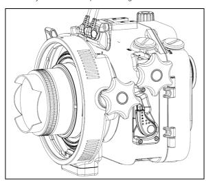
2. Mount the lens (with gears attached) on the camera.
