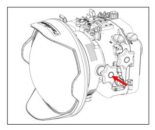
5. Engage the focus gear on the lens by pushing the knob inwards, then turn the knob both ways to check if the lens is functioning
