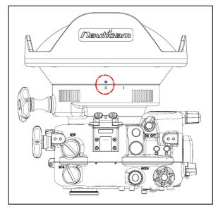
3. Turn the port count clockwise until the white dot on the adaptor aligns with the white dot on the port.
