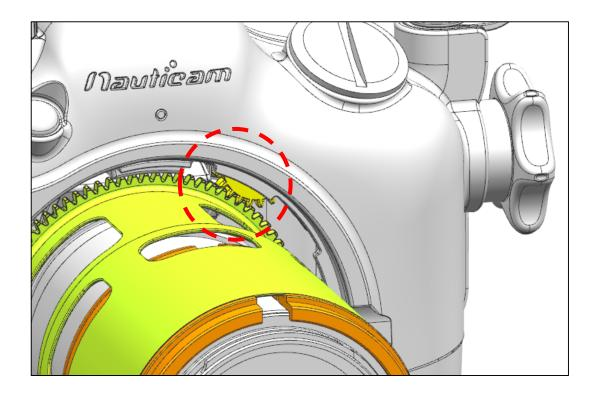
1. The SGE105-F Focus gear can be controlled by zoom/focus knobs of the housing.
