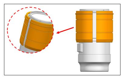
1. Insert the plastic C-rings as shown and place it over the lens.
