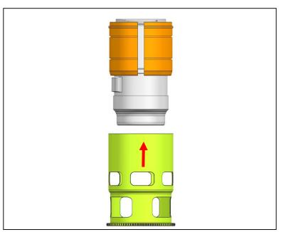
2 Insert the Focus Gear on a plastic C-ring until it reaches the flange of the plastic C-ring.
