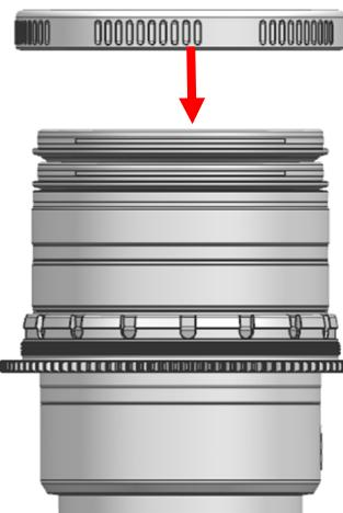
2. Place the Locking Ring over the gear, and screw it into the thread on the gear.
