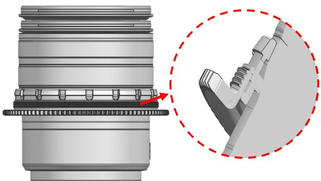
1. Insert the CR1435-Z\_Zoom Gear as shown and place it over the lens.
