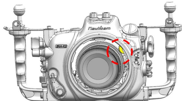
1. The CR1435-Z\_Zoom Gear can be controlled by zoom/focus knob of the housing.
