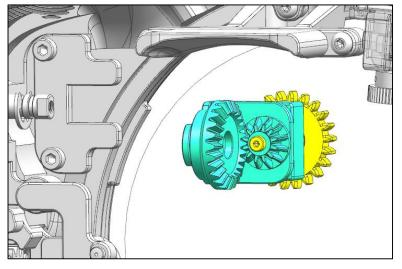
2 After take out the zoom/focus gear assembly from the shaft on the housing, remove a screw and a gear yellow-highlighted as shown.
