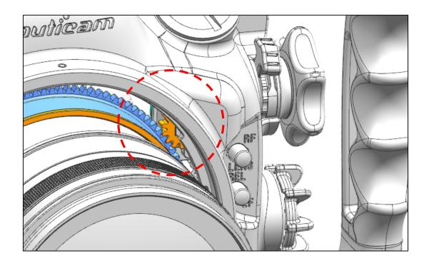
1. The CR2870-Z Zoom Gear can be controlled by zoom/focus knob of the housing.
