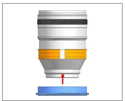
2 Insert the CR2870-Z Zoom Gear on the plastic C-ring until it reaches the flange of the plastic C-ring.
