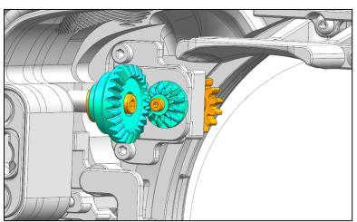
Place a gear provided to the zoom/focus gear assembly as shown, and reinstall the assembly on the housing with screws(M2 and M3) provided.
