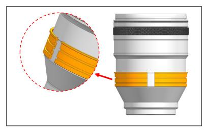
After remove rubber rings of the zoom control on the lens, Insert the plastic Cring as shown and place it over the lens.
