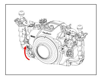
2. Lock the port into place by turning the port locking lever to the inward position. To ensure that the port is securely mounted, confirm that the green line on the safety button of the port locking lever is visible.
