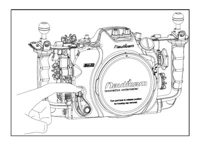
1. Push the safety button of the port locking lever downwards.
