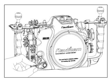
2. Turn the port locking lever to the release position as shown
